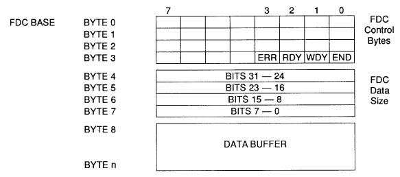
The download or upload of data utilizes FDC memory. FDC memory is a shared memory area that can be accessed by both the VX4820 and from the VXI bus. The first 4 bytes in the FDC memory are control bytes, the next 4 bytes indicate actual data size, and the rest of the memory is the data buffer. FDCBASE is required to be word aligned.
