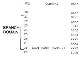
In the above example, an SEQ: BRANCH PASS command has been placed on Sequence 28. The prior seven sequences must be executed sequentially to ensure correct branch operation. It is not legal to branch to sequences 22 — 28. Any pin function may be programmed on sequences 21 — 28.
